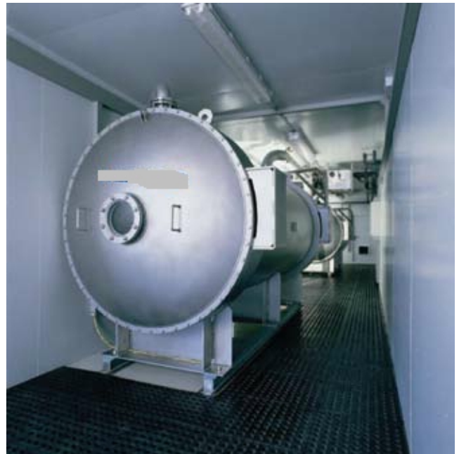
▲ Containerized ozone generator for 8,500 lbs/day
