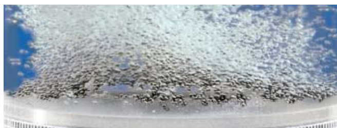
▲ OZONE INTRODUCTION: Once introduced into water ozone breaks pollutants down by oxidation
