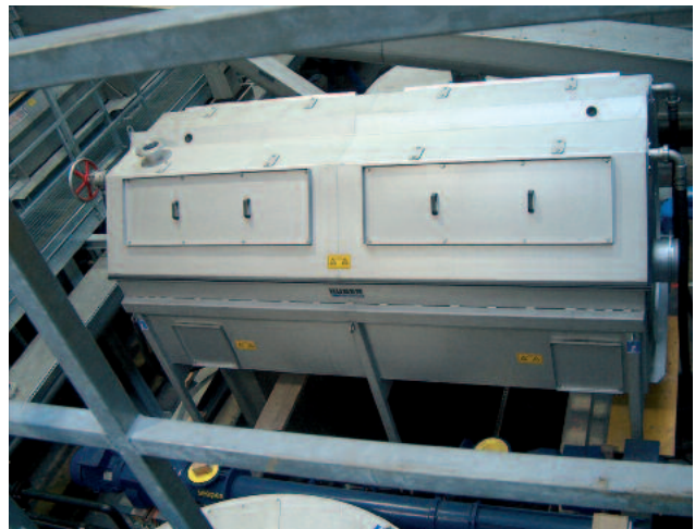
ROTAMAT® Rotary Drum Screen RoMesh® with 0.5 mesh size for wash water recovery
