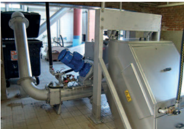
STEP SCREEN® Flexible SSF combined with HUBER Wash Press type SL for intensive screenings washing. Totally enclosed, odour-free design.
