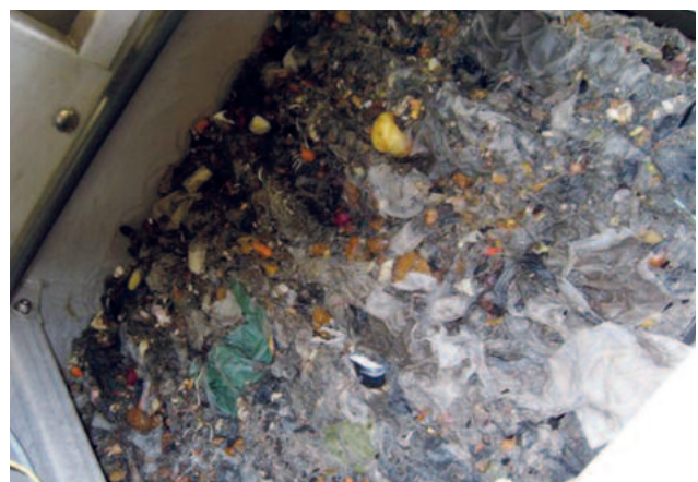
STEP SCREEN® Flexible SSF: high separation efficiency due to the narrow slot width and the produced screenings carpet, self-cleaning effect due to a moveable lamella unit
