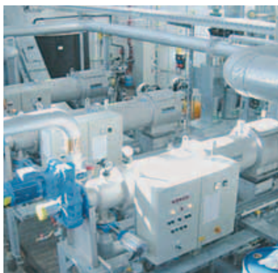
Screening of fermentation sludge (industry)
