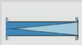
Low pressure-drop suction filter.
