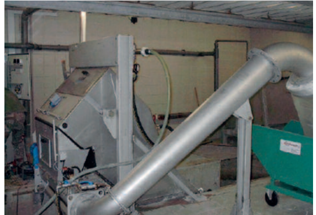
STEP SCREEN® Flexible SSF with Wash Press for optimal separation and dewatering results. Acid treated in a pickling bath for corrosion protection.
