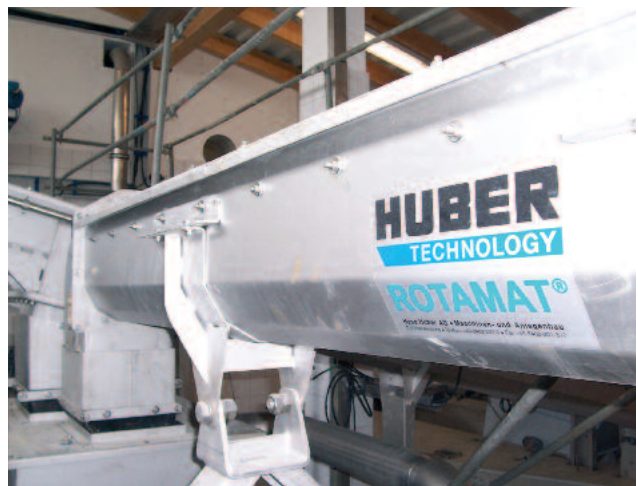
ROTAMAT® Screw Conveyor Ro 8 / Ro 8t, applicable for any type of screenings transport
