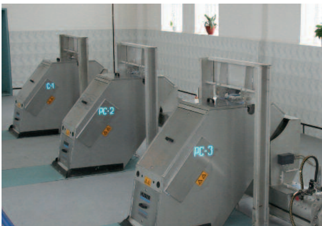
STEP SCREEN® Flexible SSF application in Russia: pivotable in the channel without having to remove the downstream HUBER Wash Press and Screw Conveyor
