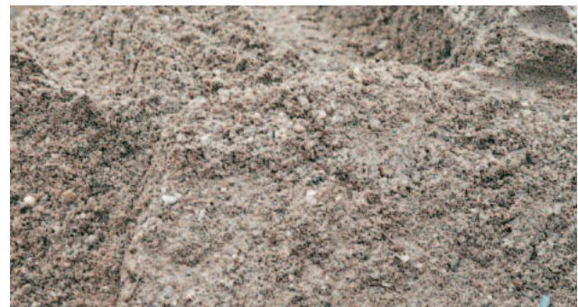
Washed grit removed at a wastewater treatment plant
