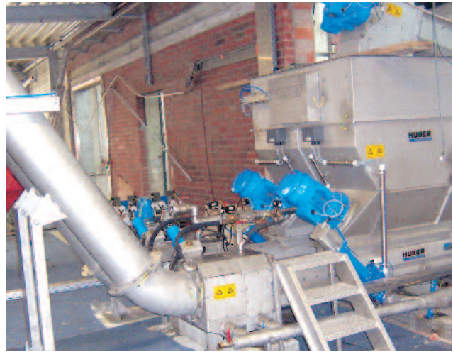
The HUBER Screenings Wash Press WAP/SL/HP for optimal screenings treatment
