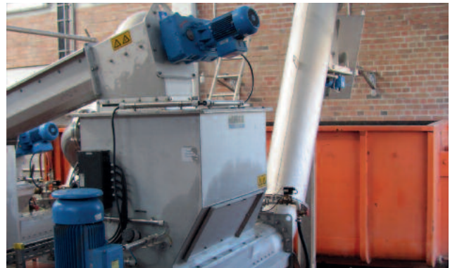
HUBER Wash Press WAP fed by a ROTAMAT® Screw Conveyor Ro 8t for a dewatering performance up to 45 % DR
