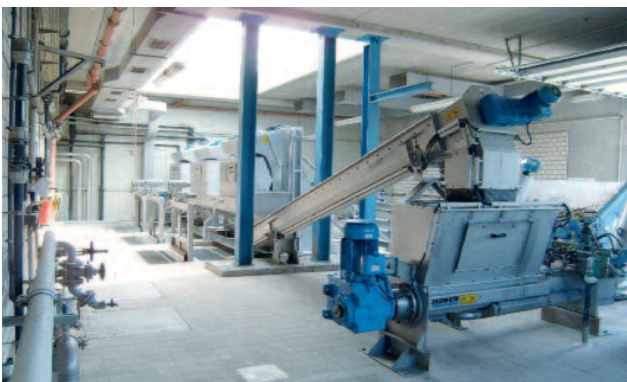
3 STEP SCREEN® Flexible SSF units and HUBER Wash Press WAP-HP with automatically controlled hydraulic counter-pressure unit for up to 60% DR
