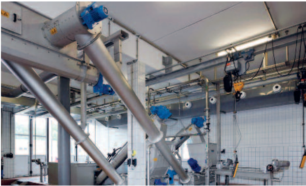
HUBER Wash Press WAP-SL treating the screenings from a HUBER Rotary Drum Fine Screen Ro 2, high-efficiency screenings washing for optimal carbon return
